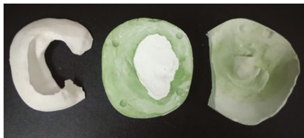
Fig. 7. 3-piece mould to process the silicone
